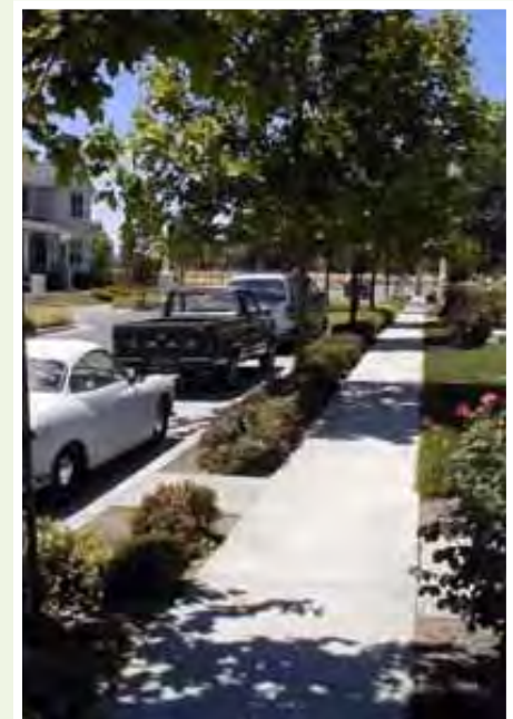
Clearly delineated and obstacle-free through zone in a residential area with a landscaped buffer and landscaped setbacks on either side are encouraged.
