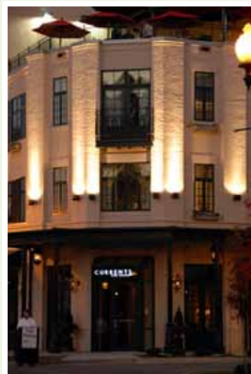
Accent lighting may be used to highlight significant architectural features of a building, enhancing its overall appearance at night.
