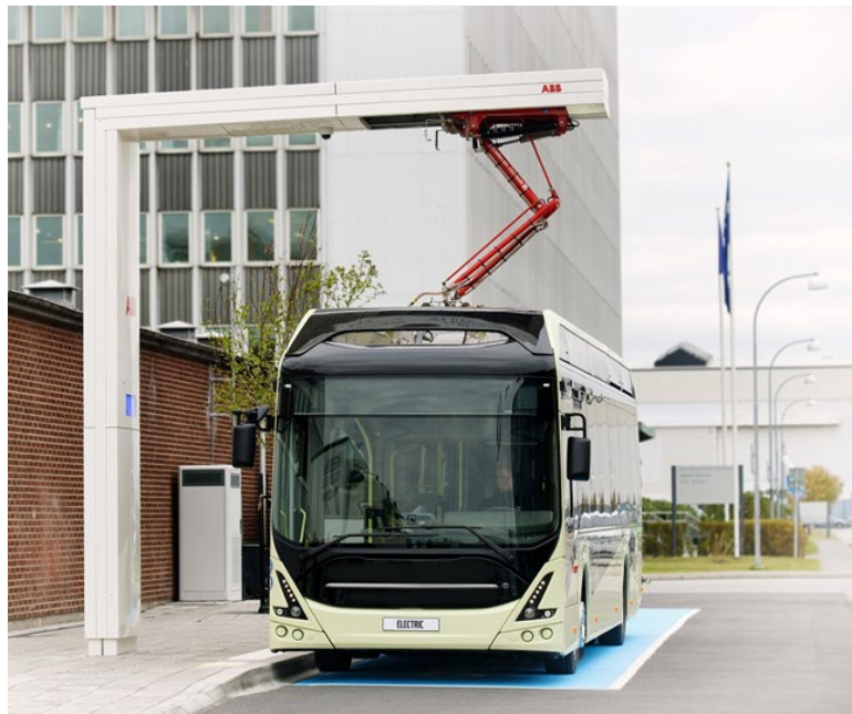
Figure 5-16 Example Overhead Charger Built by ABB
