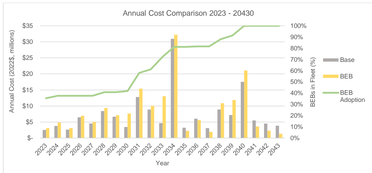
Figure 46: Annual Cash Flow for the Base and BEB Cases (bars) and BEB Fleet Composition (green line)
