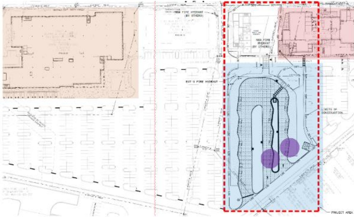
Figure 20: Bus bays limited by size of vehicle at Shipwatch Square
