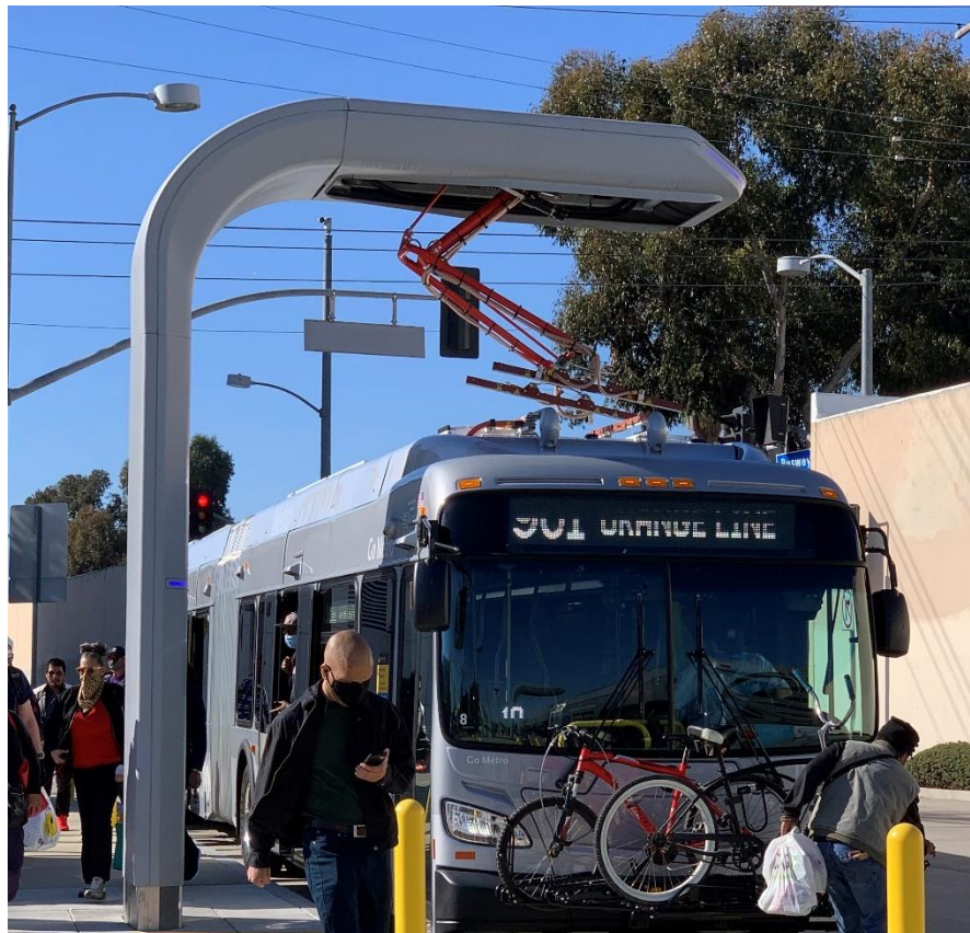
Figure 11: Overhead pantograph charger lowering onto a BEB for opportunity or on-route charging. (Metro, Los Angeles).
