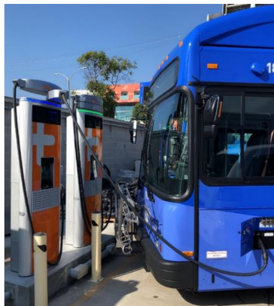
Figure 3: BEBs with pedestal-mounted plug-in chargers at UCI 5 (left) and Santa Monica BBB (right)
