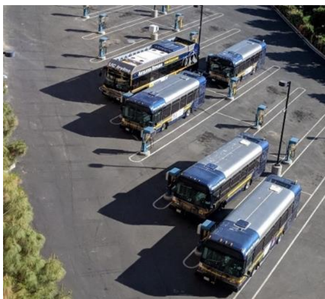
Figure 3: BEBs with pedestal-mounted plug-in chargers at UCI 5 (left) and Santa Monica BBB (right)
