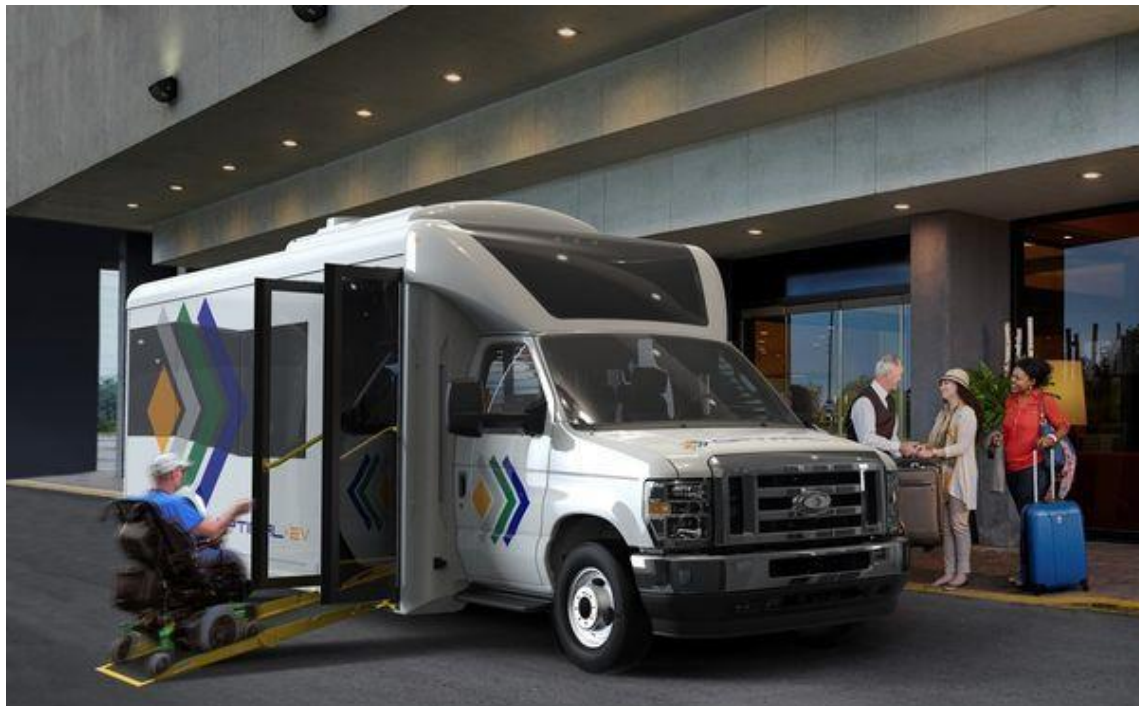
Figure 19: Optimal-EV low-floor cutaways bus using Proterra battery system
