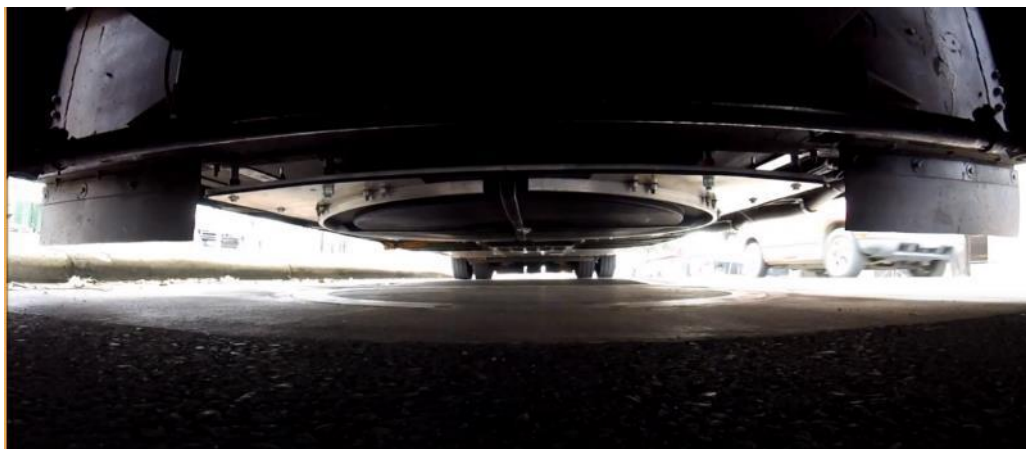
Figure 15: BYD bus fitted with WAVE charger in position to receive a charge
