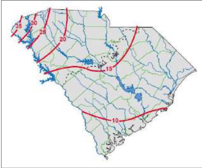
Figure 5. Average annual water yield (precipitation less evapotranspiration), in inches, 1948-1990. Source: SCDNR-Hydrology/Geology Map 2, R.N. Cherry, A.W. Badr, and Andrew Wachob, 2001.
